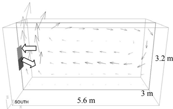
Figure 3. Configuration of the office and flow pattern
