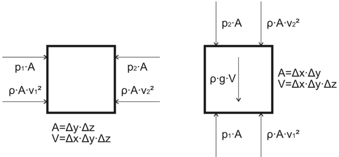
Figure 1. Forces acting on a flow element
