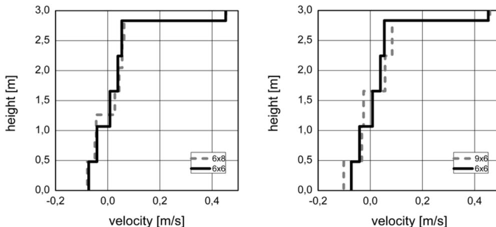
Figure 4. Influence of discretization, 3 m from inlet,  $f_{\text{loss}}=0.01$
