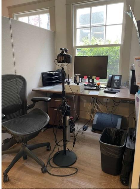
*Figure 3 - Visual and thermal comfort measurement apparatuses deployed on site.*
