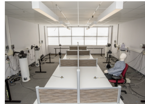
Each row of LED fixtures dimmed separately to meet illuminance setpoint
