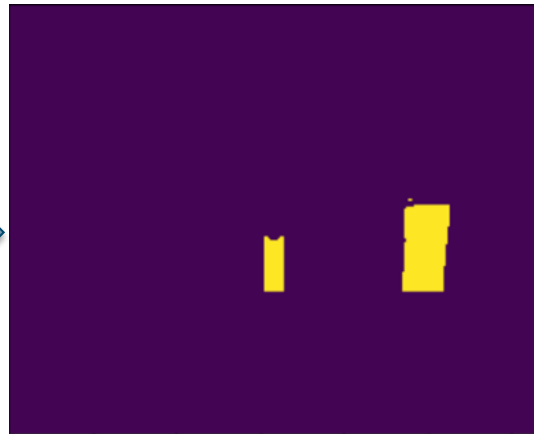
Detected thermal anomalies after applying the binary thresholding and morphological image processing
