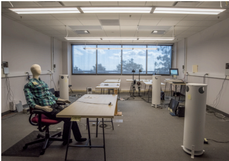
Figure 35. Photo of Licor photosensor array on desks in test cell
