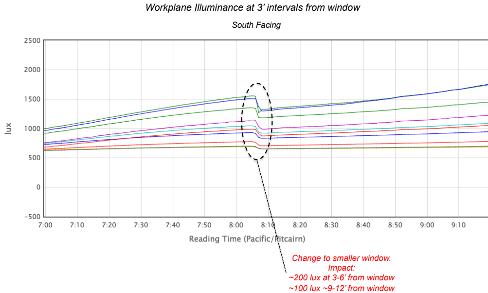
Figure 25. Impact of reducing window-to-wall ratio from 0.4 to 0.3.
