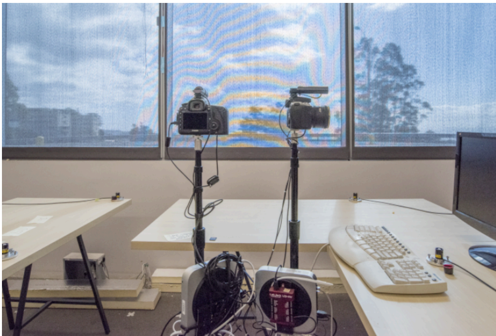
Figure 42. Photo of HDR camera, sensor, and processor packages for glare analysis in FLEXLAB
