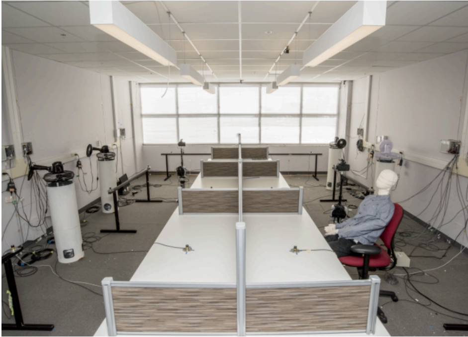
Figure F-4: The Licor photosensors are arrayed in the test space along a grid covering the desks and on the stands visible on either side of the workstations
