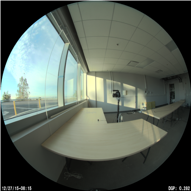
Figure F-9: Example of a false-color image from the HDR camera set-up that provides a luminance map of the camera's viewing angle. This particular HDR camera is positioned at the rear of the test cell, facing the window wall, with the pixel of highest luminance labeled.
