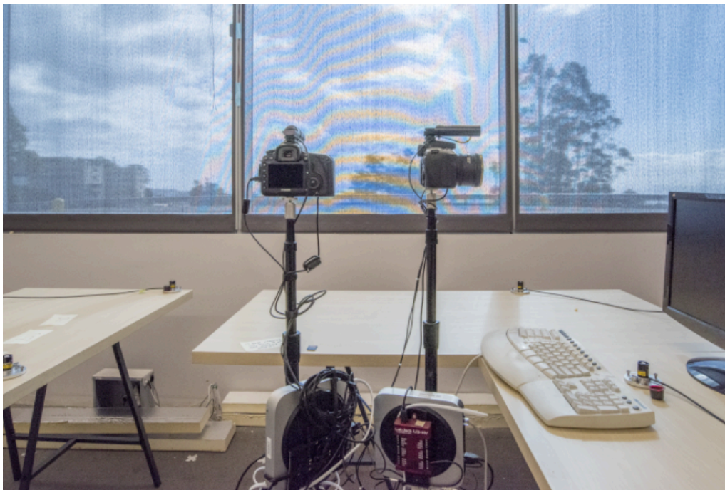
Figure F-5: Example setup of HDR camera, sensor and processor packages for glare analysis in FLEXLAB
